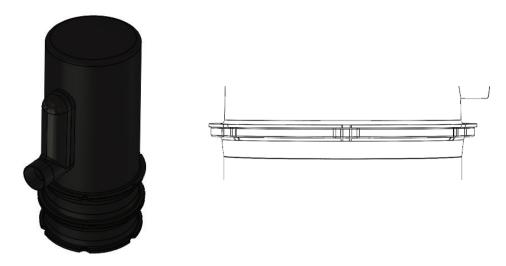
**iii.** Use the provided self tapping screws (4) to secure the grease trap to the riser. Screw through the underside of the grease trap into the riser.
