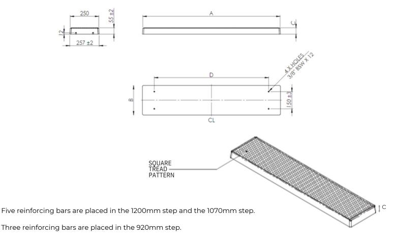
Reinforcing bars are 8mm deformed rods,
